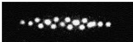
**Figure 2** The snapshot of  $^{40}\text{Ca}$  ions in the ion Coulomb crystal taken with a camera.
